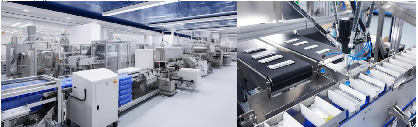
(d) Pharmaceutical packaging line consists of aspects of inspection, filling and labelling, carton and cardboard box packaging Figure 1 Examples of packaging machines
