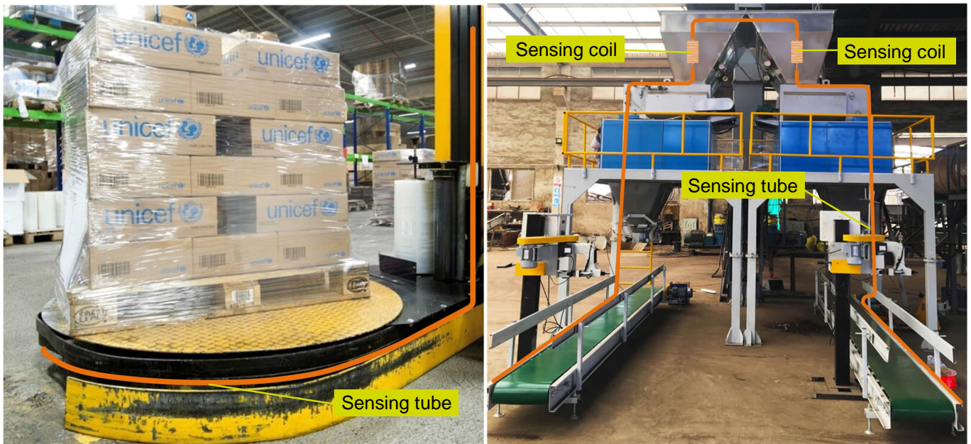
(b) Illustration of ADW sensing tube placement in packaging machinery (left) and object protection using sensing coils (right) Figure 3 SecuriHeat ADW placement in production line machinery (risk-based local detection)
