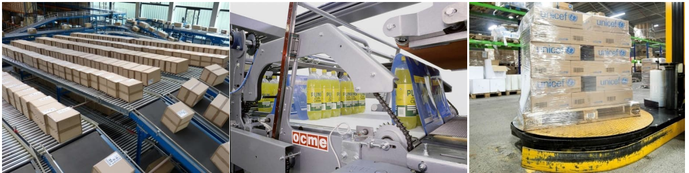
(a) Common packaging production line: box/carton machines (left), wrapping and sealing (middle), packing and palletising (right)
