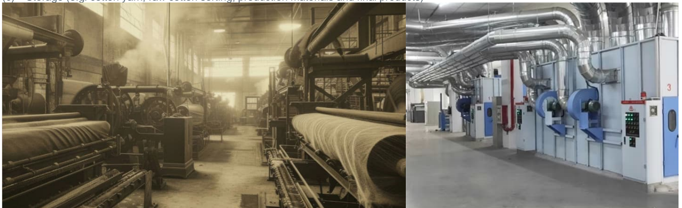
(d) Hazardous environments with combustible dust and fibres in dusty operation environment (left) and spinning mill dust filters (right)
