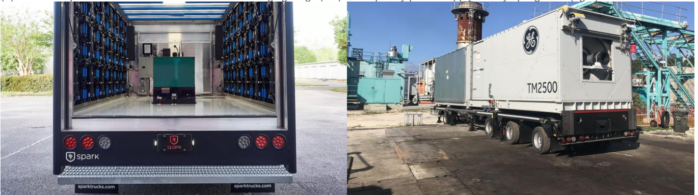
(c) Trailer-based power generator/plant (used for oil field power, remote power, and emergencies such as natural disasters)
