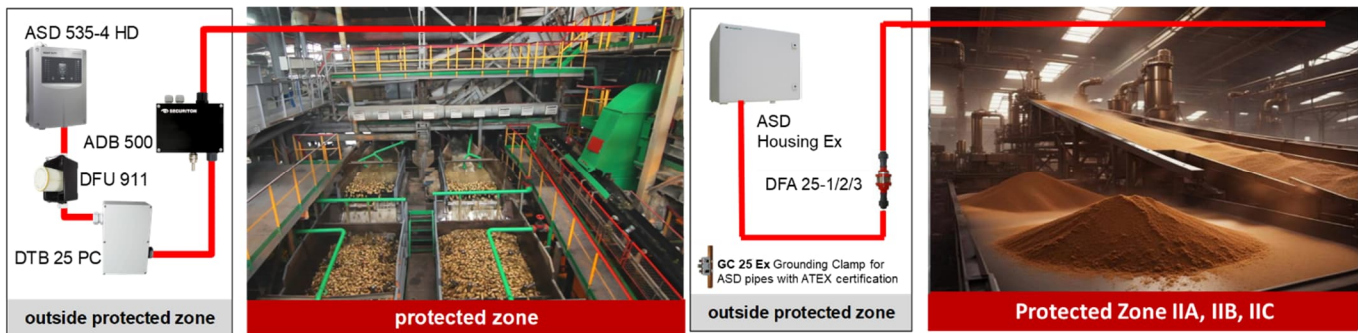
(d) High IP rating enclosure and very dusty environment (e.g., sugar plant) or classified hazardous areas (spices processing)
